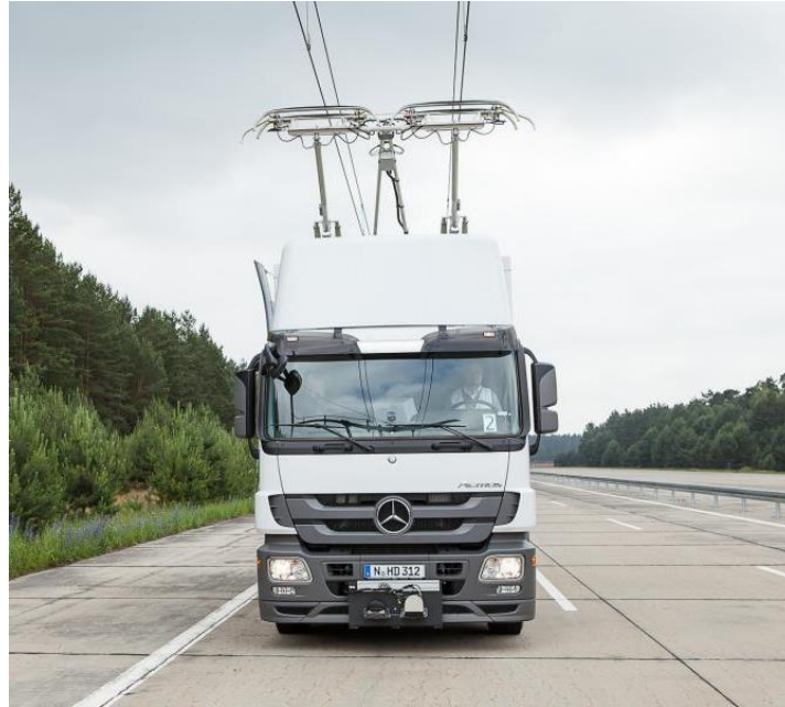
Figure 18 - A trolley truck being tested in USA by Siemens (image from www.welt.de )
